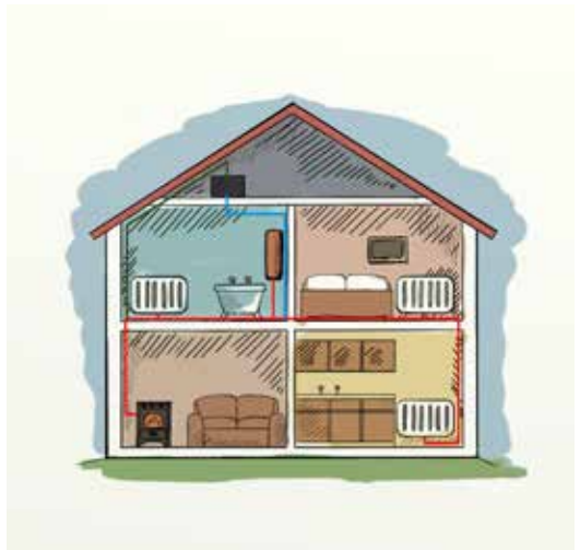
A boiler stove is plumbed into your central heating system
